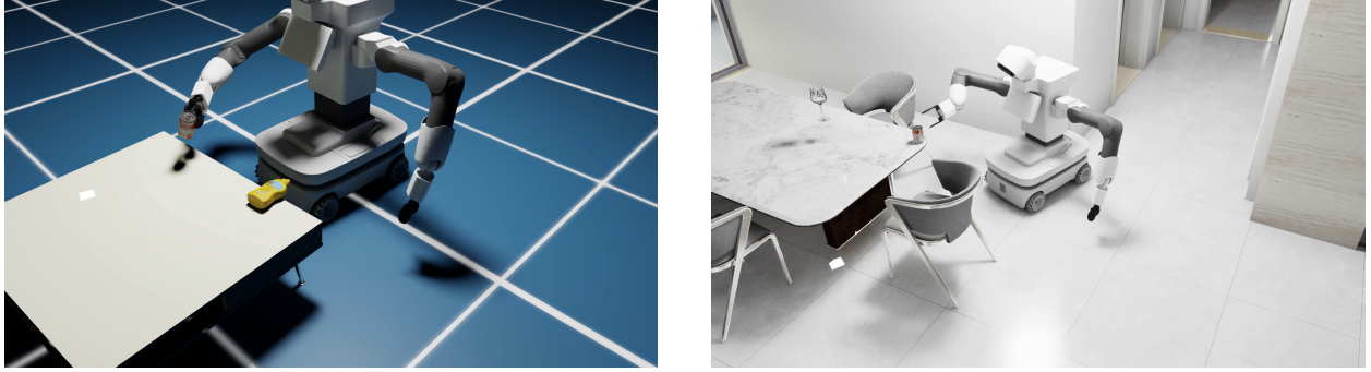
Figure 4: Evaluation environments used in the report. Left: simple scene used for baseline ACT training and evaluation. Right: photorealistic indoor apartment scene used for transfer, adaptation, and integrated system testing.
